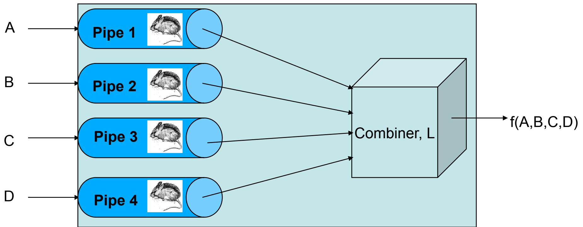
Inside the black box: Pipes *isolate* input streams, then combine
